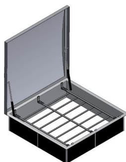
Application example for opening skylight.
